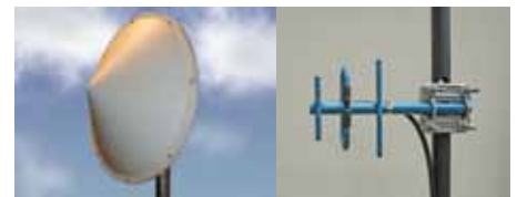
Parabolic and yagi antennas are also used for smart grid remote monitoring and control
